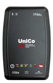
The name UniCo brings together the terms **Uni**versal **Co**nnecting and is a multifunctional device with multiple functions. Compact, lightweight, characterized by maximum flexibility of use and good autonomy, it is designed for two main purposes: to receive T1 / C1 mode wM-Bus messages in the 868MHz ISM band and to interface to program Maddalena devices.
