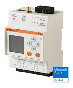
RTUEVO1T (1.ETRSEQ.0051) is a datalogger for the acquisition of data from 1.ETRSEQ.0012 repeaters that collect information from wired and wireless M-Bus compliant devices, such as meters, cost allocators and sensors, via a MESH network. The device can handle up to 3000 meters (2500 wireless + 500 wired) and can store daily readings for 10 years.
