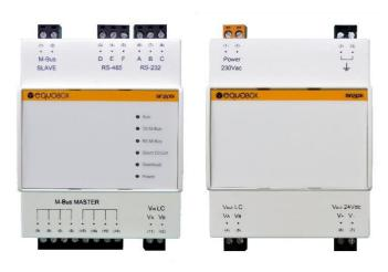
The M-Bus level converter 1.ETRSEQ.0006 allows interfacing to a network of M-Bus compliant devices (EN13757-2 Physical Layer) and supports up to 250 slaves\*.
